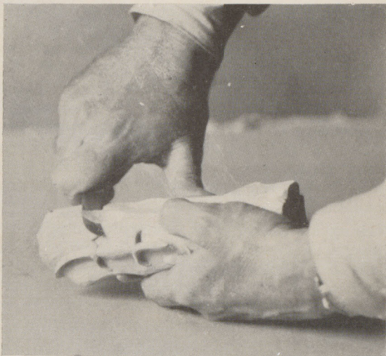
Plate 6. Holding the knife for making inward cuts.
