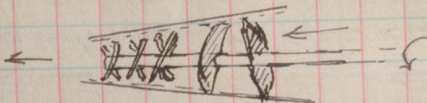
The rollers & presses externally somewhat like this. half circles of slant iron fixed to the shaft, the throes smaller in pairs, & all arranged so as to form parts of sphere plane, forcing the material steadily forward in turning.
