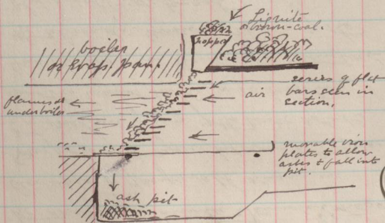
N.B. The series of flat grate bars are drawn as being too steep a slope. The stoker clears the bars from time to time & sets the fuel in instead toward the ash plate by introducing a pointed iron. Any clinker forming is thus easily removed.
