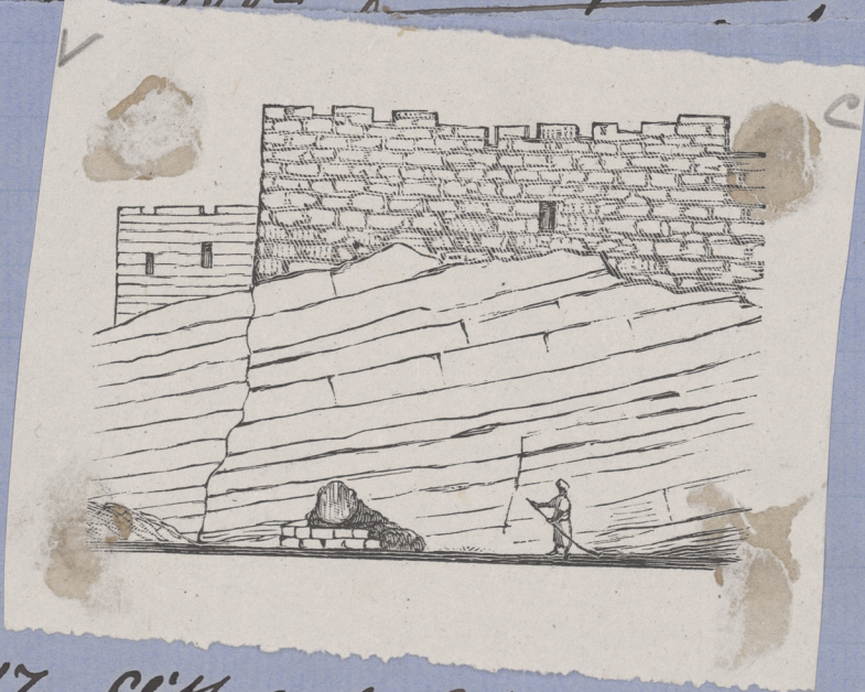
Fig 17. Cliff and City wall, at the entrance of the Royal Quarries, showing the dip of the limestone.
